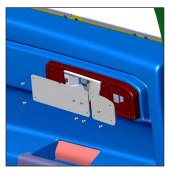
Position the Cover Plates over the Door Handle and the Lock.
