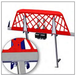
Align the slots of the Cargo Barrier Brackets to the "previously loosen" bolts of the Top Bar Assembly.
