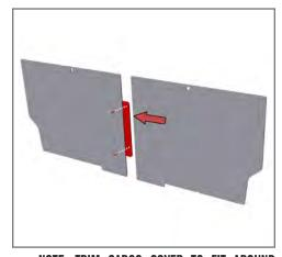
NOTE: TRIM CARGO COVER TO FIT AROUND CARGO BARRIER VERTICAL SUPPORTS. SEE DIAGRAM ON LAST PAGE.
