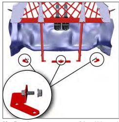
30. From the cargo compartment of the vehicle attach the retractable belt to the center anchor point located on the Floor Bracket and the outboard seat belt on the DS/PS Tongue Bracket.
