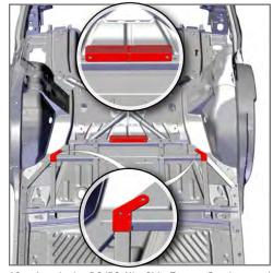
Attach the DS/PS Hip Side Tongue Brackets and with previously removed OEM hardware.
