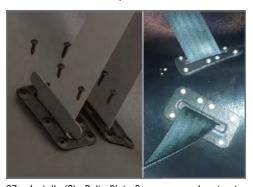
Install (2) Belt Slot Covers around retractor webbing using built in cutout in Belt Slot Covers.
