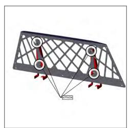
Attach the Cargo Barrier Brackets to the Cargo Barrier with provided (4) 1/4-20 Socket Head Cap Screws.
