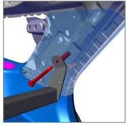
14. Tilt the Top Bar Assembly forward and insert the (2) 2.5" Spacers into the C-pillar trim securing with (2) 10 mm x 90 mm bolts.
