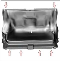
Secure the front face of the ABS Seat to the 0EM seat frame structure with provided (4) #14 1 1/2" Tek Screws.
