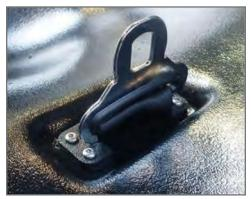
Place the Tooth C-Retainer on webbing on outboard seatbelt and outboard slot so that it pinches webbing and closes gap around webbing.
