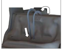
25. Attach the RED Ring Buckle to seatbelts.
