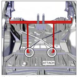
Insert the Frame Assembly into vehicle and lightly secure in place with previously removed OEM hardware.
