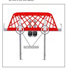
18. Secure the bottom of the Cargo Armor Brackets to the Top Bar with (2) #14 x 1" Tek Screw.
