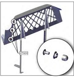
Secure the DS/PS Side Wings to the rear of the Cargo Armor with provided (6) 1/4-20 x 1/2 Carriage Bolts, 1/4-20 Flange Nuts and Nut Covers.
