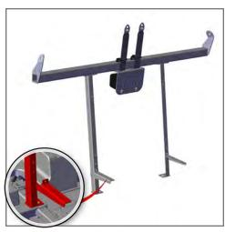
Pre-assemble the Seat System Frame by attaching the Lower Seat Supports to the DS/PS legs using (4) 1/4" x 1/2" bolts.
