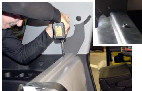
Go to back side of seat through cargo area. Attach hip tongue on top of frame leg supports. Attach seat to frame assembly by screwing through seat top flange into tube of frame assembly. Using (2) #14 x 1.5" hex head self-drilling screws, attach seat to top of frame. Locate screws about 8" from either end of frame.
