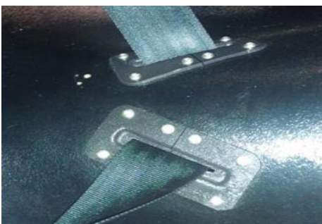
Install seat belt slot cover around retractor webbing using the built in cutout in the belt slot cover. Cutouts should face toward center. Secure belt slot cover to seat with (14) #6 x 0.625 sheet metal screws.
