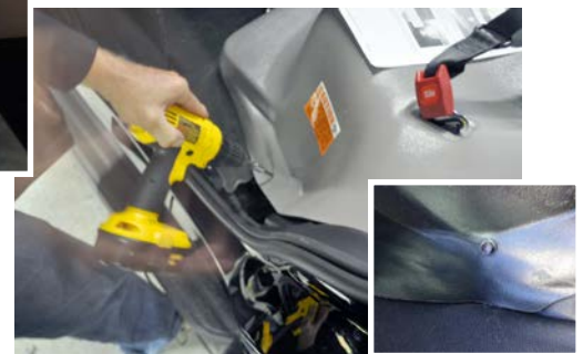
Use (2) #14 x 1.5" hex head self drilling screws, attach bottom of seat to floorboard. Screws will need to go in pre-made holes on bottom of seat.
