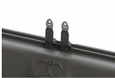
Pull the retractor webbing through slots at top of seat and through webbing swivel. Install webbing swivels to seat and top bar using (2) 7/16 flange bolts.
