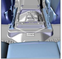
2. Move front seats completely forward and loosen the rear inside T-50 bolts.
