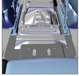
3. Push the seat up slightly to slide the front legs of the GR6 Base under seat rial, between rail and vinyl/carpet flooring.
