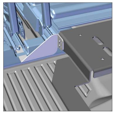
4. Loosen the rear seat inside T-50 bolt and insert the P/S Rear GR6 Leg between the rail and flooring. Secure the Leg to the GR6 Base with provided button head cap screws.
