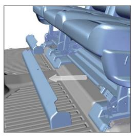
1. Adjust/slide rear seats fully backv. Pull to unclip plastic trim from rear seat frame.
