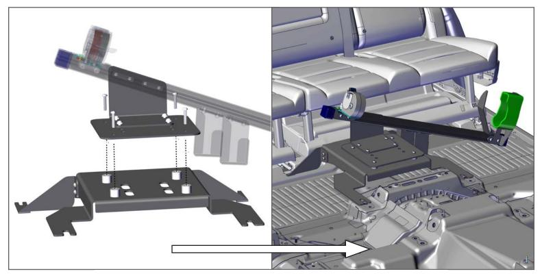
6. Secure the Offset Base Plate to the GR6 Base with provided spacers and 5/16 x 1.5 button head cap screws. Insert the assembled backbone and secure the Angled Bracket to the Offset Base Plate with provided hardware.
