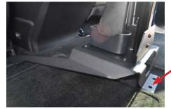
Slide GR6 mounting plate on top of inside seat rails of front seats. Mark hole location for rear of mounting plate for AVK install. Remove mounting plate and set aside.
