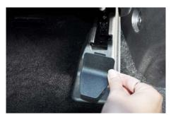
Remove cap from inside back seat rails of front seats and loosen (2) 13mm seat bolts on rear of front seats nearest the console.
