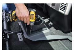
Position assembled backbone onto GR6 mounting plate.
