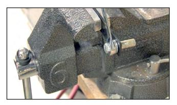
4. Use 9/16" box end wrench to secure the flange nut.
