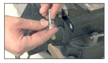
Place 5/16-18 x 1.5" long bolt through the 3/8" flange nut and hand thread bolt into the AVK Fastener.
