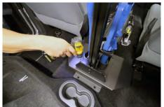
Position assembled backbone onto GR6 mounting plate.
