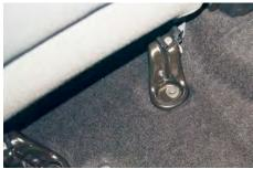
Remove (2) 18MM seat bolts on rear of front seats nearest transmission hump.
