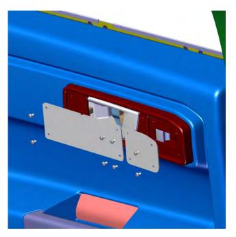
1. Position the Cover Plates over the Door Handle and the Lock.
