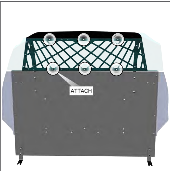
IF ORDERING THE POLY COVER - 475-1709 10. From rear seat of vehicle, use (16) carriage bolts and flange nuts to attach the Poly Cover to the front of the Secure Grid and Support tubes.
