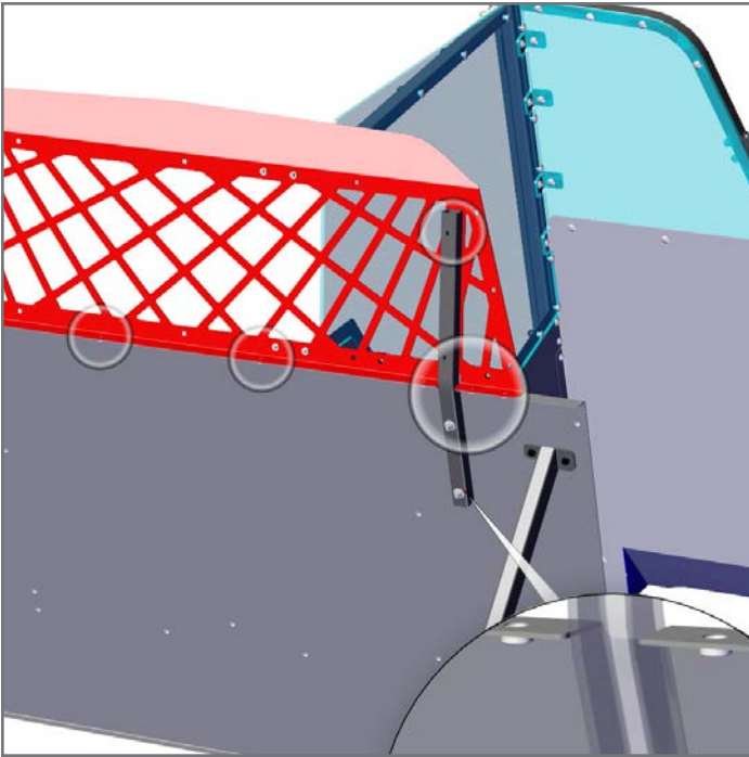
25. From cargo side of vehicle, attach the pre-assembled Secure Grid assembly to the Steel Panel with hex bolts and washers and Support Tubes with (4) carriage bolts and flange nuts.
