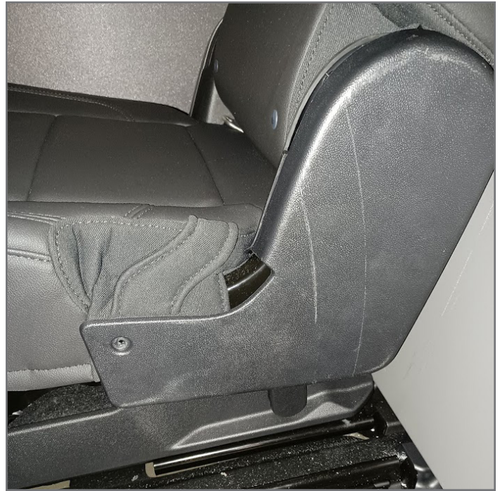
12. Fold down and tilt up the D/S rear seat. Remove the OEM screw and pop loose the inside side trim of the P/S rear seat. Trim not reinstalled.
