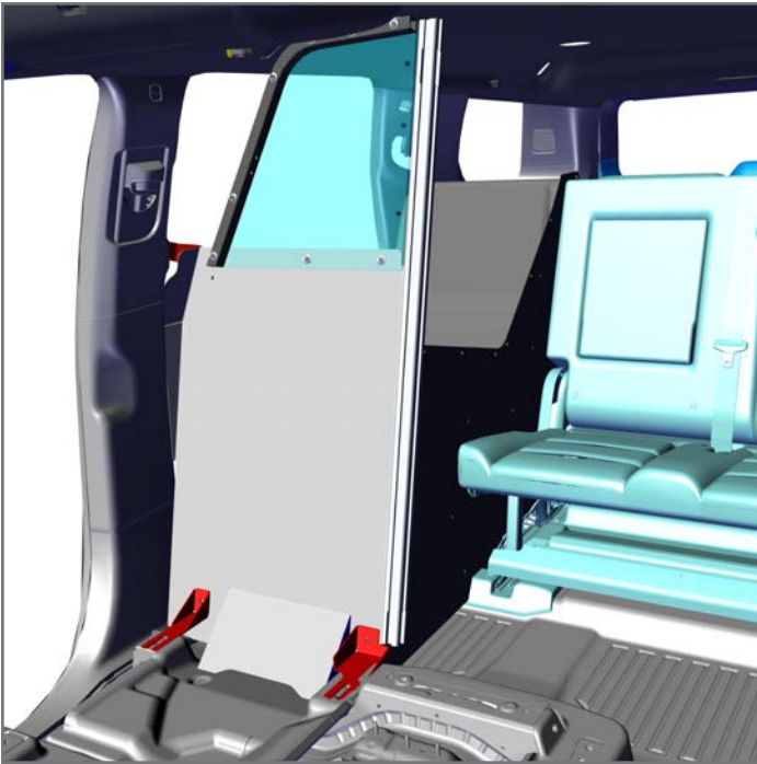
17. Install Assembled Front Divider into vehicle. This will require a little twisting to get into proper position. Bolt down Foot Mount Brackets to Assembled Front Divider with provided carriage bolts and flange nuts.
