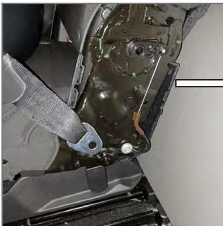
14. Using a T-47 socket, remove the OEM seatbelt buckle on the inside of the P/S rear seat. Insert the provided Seat Belt Extender through the slot of the ABS Seat. Install ABS Seat into the vehicle and secure the Seat Belt Extender to the previously removed OEM seatbelt location.
