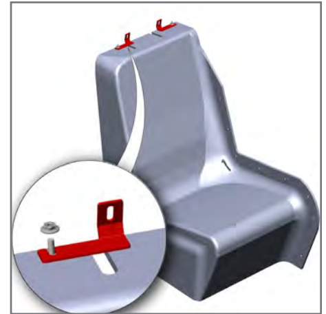
13. Loosely attach the ABS Seat Brackets to the ABS Seat with provided carriage bolts and flange nuts.
