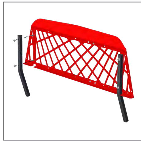
23. Outside of vehicle, attach the Secure Grid to the Support Tubes with (4) carriage bolts and flange nuts.
