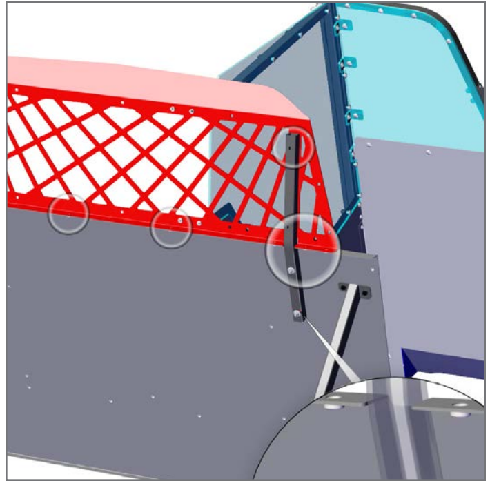
20. From cargo side of vehicle, attach the pre-assembled Secure Grid assembly to the Steel Panel with hex bolts and washers and Support Tubes with (4) carriage bolts and flange nuts.
