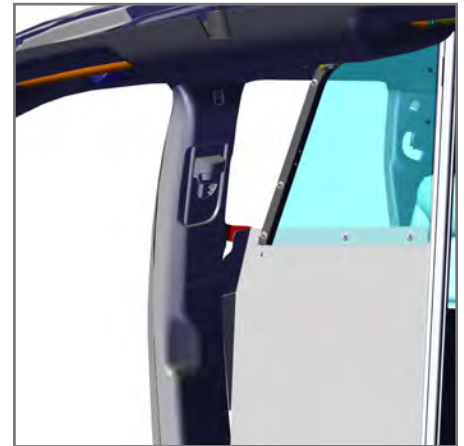
13. Install Assembled Front Divider into vehicle. This will require a little twisting to get into proper position. Bolt down Foot Mount Brackets to Assembled Front Divider with provided carriage bolts and flange nuts.
