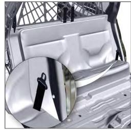
12. Pull the Hip Side Tongues Belts through both driver and passenger side slots of the ABS Seat.
