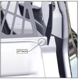
15. Use (2) #14 x 1 1/2" self-tapping screw to attach the top of the ABS Seat to Top Bar Frame.
