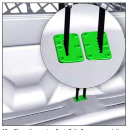
Place the center Seat Belt Covers around the previously installed seat belts. Align the Seat Belt Covers to the slots in the ABS Seat, attach with provided (14) #6 x 5/8 sheet metal screws.
