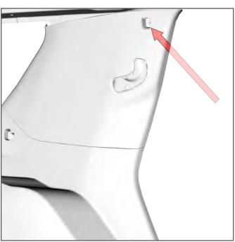
Remove the upper C-Pillar trim by popping out square trim cover, giving access to the 9/32" screw at the top of the headliner.
