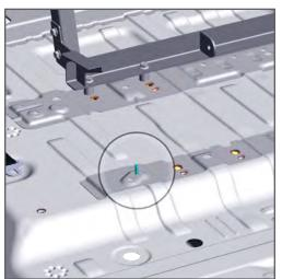
10. Remove the plastic alignment stud on the passenger side floor.
