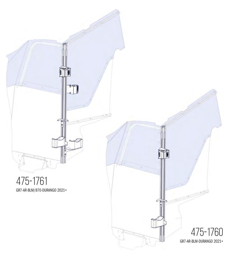
1. Button Head Cap Screws will already be attached to T-Block and Mounting Brackets. Loosen the screws slightly.
