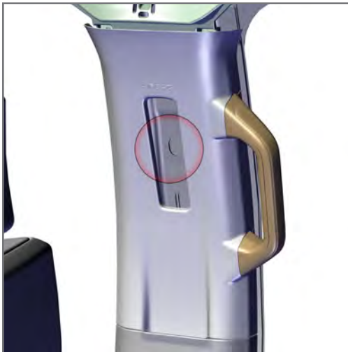
3. Remove plastic caps from the P/S and D/S B-Pillar seat belt adjusters. Use a T-45 socket to remove the OEM Torx screw.
