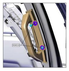
4. Remove the (2) 7 mm screws attaching the B-Pillar handle.
