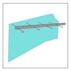
Outside of vehicle, attach the Stiffener Tube to the D/S Upper Poly Center Divider with provided carriage bolts and flange nuts.
