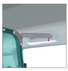
Loosely attach Headliner Handle Bracket onto the headliner hook location. Reuse OEM Torx screw.
