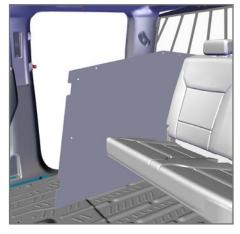
7. Slip the Lower Steel Center Divider between the split in rear seats.
