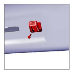
Remove cover from P/S headliner hook exposing the (1) T-20 Torx screw. Remove screw and set hook aside.
