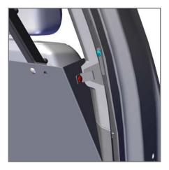
Loosely attach B-Pillar Bracket onto Assembled Front Divider. Use provided carriage bolt and flange nut.
