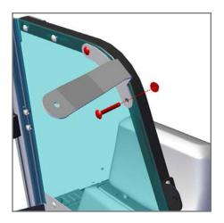
Loosely attach Headliner Handle Bracket onto Assembled Front Divider. Use provided carriage bolt and flange nut.
