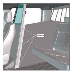
Loosely secure Lower Steel Center Divider onto Assembled Front Divider using provided carriage bolts and flange nuts.
