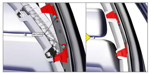
5. Using the previously removed OEM hardware, attach the provided B-Pillar Bracket and B-Pillar Cover Bracket. Re-attach B-Pillar trim and seat belt adjuster at this time.
