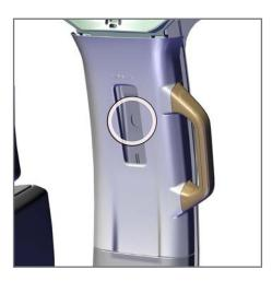
Remove plastic cap from the P/S B-Pillar seat belt adjuster. Use a T-45 socket to remove the OEM Torx screw.
