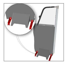
Outside of vehicle, attach Inner Foot Mount Brackets to Assembled Front Divider using provided carriage bolts and flange nuts.
