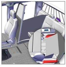
Install Assembled Front Divider into vehicle, slipping the Foot Mount Brackets under the previously loosened OEM seat bolts, this will require a little twisting to get into proper position.
