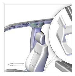
Slide P/S front seat completely forward. Remove rear OEM trim cover to expose the 13 mm bolts. Unscrew bolts halfway.
