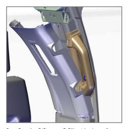
Pop the P/S upper B-Pillar trim loose from the grab handle side giving access to its mounting hardware. It's not necessary to fully dislodge trim from its position.
