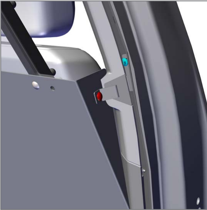
10. Loosely attach B-Pillar Bracket onto Assembled Front Divider. Use provided carriage bolt and flange nut.
