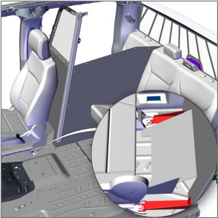
9. Install Assembled Front Divider into vehicle, slipping the Foot Mount Brackets under the previously loosened OEM seat bolts, this will require a little twisting to get into proper position.
