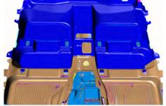
Place GR6 Mounting Plate onto transmission hump on top of inner most seat hole locations.
