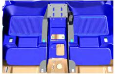
Adjust Mounting Plate to required position. Fully tighten all seat bolts to secure Mounting Plate.
