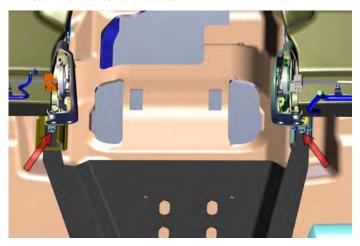
4. Replace and tighten 18mm nuts under rear seat. Roll back carpet/mat back into original place. Tighten T45 seat bolts on rear of front seats.
