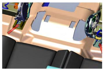
1. Loosen (2) T45 seat bolts on rear of front seats nearest transmission hump.
