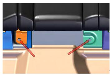
Roll the carpet/mat back towards hatch to expose nuts. Remove 18mm seat nuts under center of rear seat.
