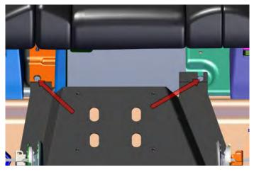
3. Slide GR6 mounting plate underneath seat rails of front seats. With carpet/mat still rolled back under rear seat place GR6 plate onto studs.
