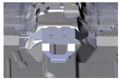
Reposition mounting plate underneath sear rails of front seats and tighten all OEM seat bolts and use provided hardware for AVK locations.
