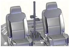
Position assembled backbone onto GR6 mounting plate.
