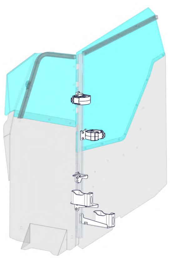
Button Head Cap Screws will already be attached to T-Block and Mounting Brackets. Loosen the screws slightly.
