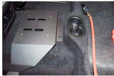
Slide GR6 mounting plate underneath seat rails of front seats Mark hole locations at rear of mounting plate for AVK install. Remove mounting plate and set aside.
