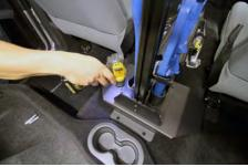
Position assembled backbone onto GR6 mounting plate.
