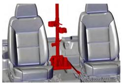
Position assembled backbone onto GR6 mounting plate.
