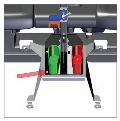
5. Position assembled backbone onto GR6 mounting plate. Secure to plate using provided (4) button head cap screws.
