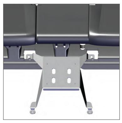
3. Set the back legs of the GR6 mounting plate into the previously remove rear seat trim sections while nesting the front of the GR6 mounting plate legs into front seat inside rear bolt hole locations.
