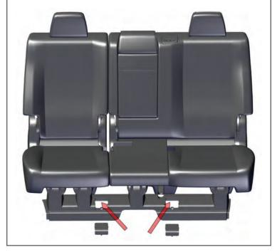
With a small screwdriver, unsnap and set aside the rear seat trim covers exposing the OEM seat bolts. Remove with a 18 mm socket.
