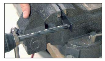
1. Drill out existing hole to 1/2" or drill new hole per installation instructions.
