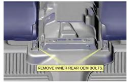
Loosen inside rear, front seat bolts nearest transmission hump.
