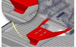
Slide GR6 mounting plate underneath seat rails of front seats Mark hole locations at rear of mounting plate for AVK install. Remove mounting plate and set aside.
