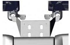
Replace and tighten OEM bolts to secure GR6 mounting plate.
