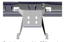
Set the back legs of the GR6 mounting plate into the previously remove rear seat trim sections while nesting the front of the GR6 mounting plate legs into front seat inside rear bolt hole locations.
