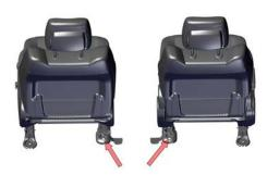
With a small screwdriver, unsnap the inside rear seat trim (of the front seats) exposing the OEM seat bolts. Remove with a 15 mm socket.
