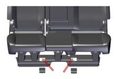
With a small screwdriver, unsnap and set aside the rear seat trim covers exposing the OEM seat bolts. Remove with a 18mm socket.
