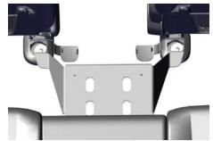
Replace and tighten OEM bolts to secure GR6 mounting plate.
