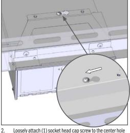
Loosely attach (1) socket head cap screw to the center hole of each previously attached Cargo Cover Bracket. Install the Gun Box under the Cargo Cover, lift-up into the Cargo Cover exposing the screw within the hole-slot. Slide over to hold in place.
