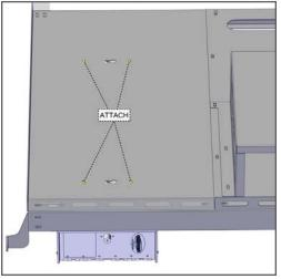
3. Attach the remaining (4) Socket head cap screws through the Cargo Cover to securely attach the Gun Box into place.
