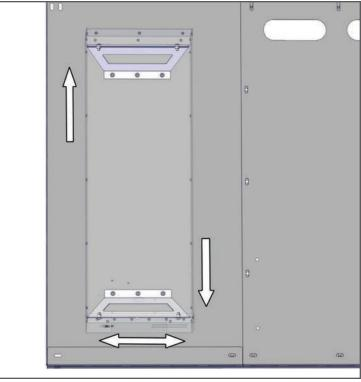
2. Adjust to desired location and mark points to drill through the (6) mounting holes located on the Cargo Cover Brackets.
