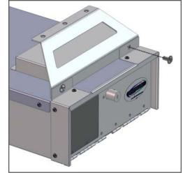
1. Attach the (2) Cargo Cover Brackets to the tabs found on top of the "Stash" Gun Boxwith (4) 5/16-18 socket head cap screws. NOTE: 3/16" Torx Socket Bit required
