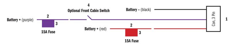
\* - Battery connection can be Switched or Constant basted on the desired function. Ignition ON or OFF function.
