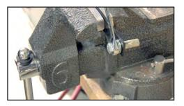
Use 9/16" box end wrench to secure the flange nut.
