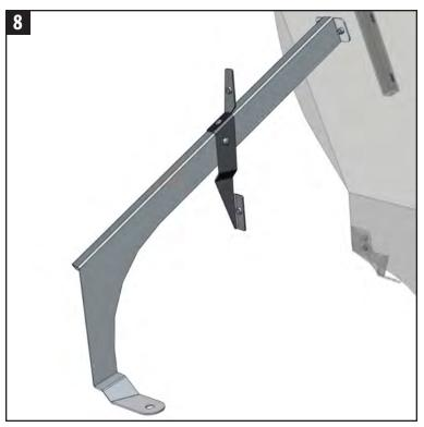
8 Attach the Rear Bracket to the Cargo Barriers Rear Leg with (2)-1/4"-20 carriage bolts and flange nuts.
