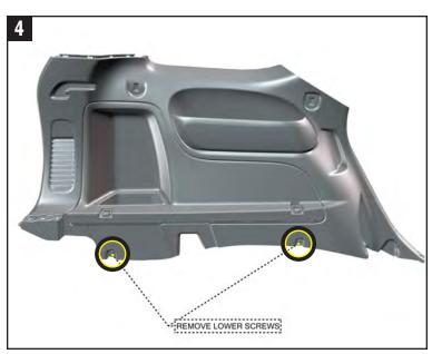
4 Remove the (2) lower screws attaching the cargo side panel to the vehicle. Pop the trim loose starting from the back working your forward giving yourself just enough room to modify the trim.
