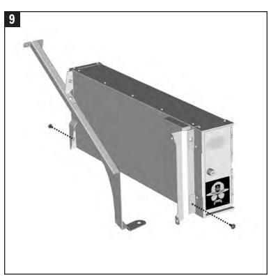
$\begin{array}{ll} \textbf{9} & \text{Complete assembly by attaching the Gun Box to the Front/Rear Brackets with} \\ & \textbf{(4) 5/16"-18 socket head cap screws. Fully secure all hardware at this time.} \end{array}$
