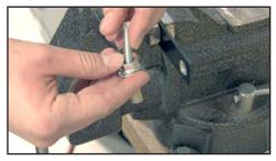
2. Place  $5/16-18 \times 1.5$ " long bolt through the 3/8" flange nut and hand thread bolt into the AVK Fastener.
