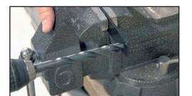
Drill out existing hole to 1/2" or drill 1. new hole per installation instructions.
