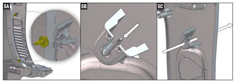
Remove the (2) clips that secure the trim. Cut the tab away from the trim support. Use the circular profile of the interior trim support to drill a 9/32" hole through the trim followed by a 3/4" inch hole.
