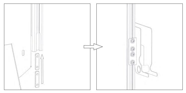
3. Remove the T-Blocks and mounting hardware from the AR Secure Bracket and slide them into the channel. Position of the AR Secure Bracket and in place and attach with the (4) previously removed Button Head Cap Screws, Washers and Lock Washers.
