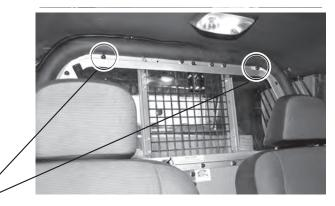
1. Start by removing the (2) Factory 1/4" nuts and carriage bolts using a 7/16" wrench or socket. Remove the ones on the top section in the outer position of window frame on partition.
