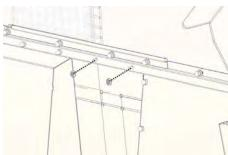
Remove two flange nuts while your helper is holding the carriage bolts in place from the back seat.
