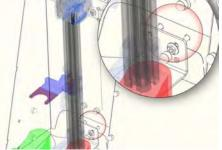
Attach the lower bracket with the provided carriage bolts and flange nuts. Secure all four mounting points and finish assembly with provided black plastic nut covers.
