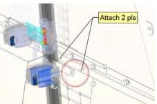
Place the gun mount assembly in the recessed area of the partition. Insert the top bracket onto the carriage bolts and secure with previously removed flange nuts.
