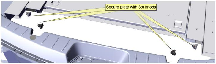
Place Spacer Cover onto opening of flooring and secure using provided (4) 3 point knobs.
