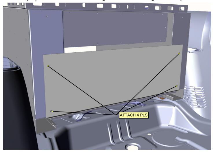
Attach Backstop onto Storage System using (4) Buttonhead Cap Screws.
