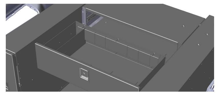
Tighten all hardware. Slide Drawer back into position
