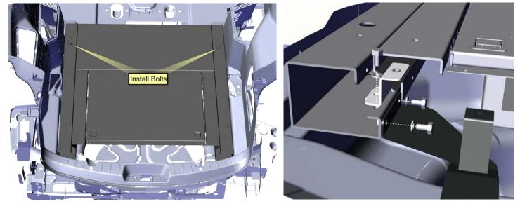
Position Storage System Flooring into vehicle and secure rear of flooring into holes of either side of flooring using (2) OEM 11mm bolts. Secure front of Storage System Flooring onto previously installed Brackets using (4) Buttonhead Cap Screws. Place provided caps on drill holes of OEM trim.
