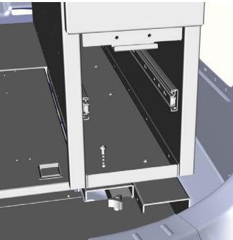
Position Towers onto Storage System Flooring and either side of access door. Secure to flooring using (6) Buttonhead Cap Screws per tower into provided openings.
