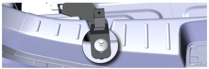
Place Brackets through OEM rear hatch door sill trim and loosely secure reusing OEM 8mm bolts.
