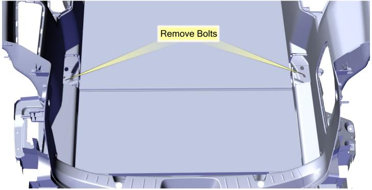
Remove (2) 11mm bolts from OEM flooring and remove flooring. (2 pieces)
