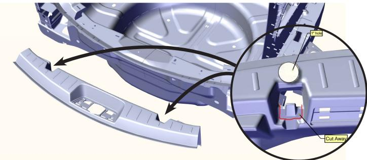
Drill 1" hole into the rear hatch door sill trim and cut/remove cargo hook on both sides. Then Remove (2) 8mm bolts.
